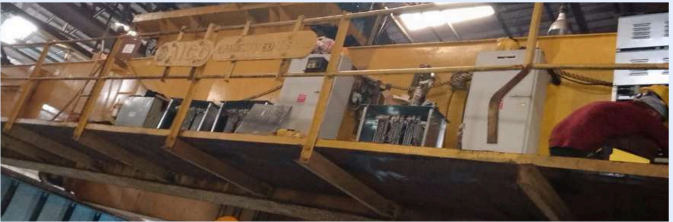
Major Refurbishment of EOT crane 10 Ton to 30 Ton @10 NOs carried out at major steel Giant
